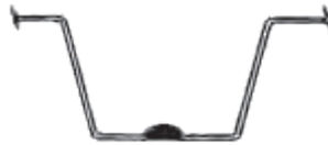
CASE 1 Weld through single sheet thickness
