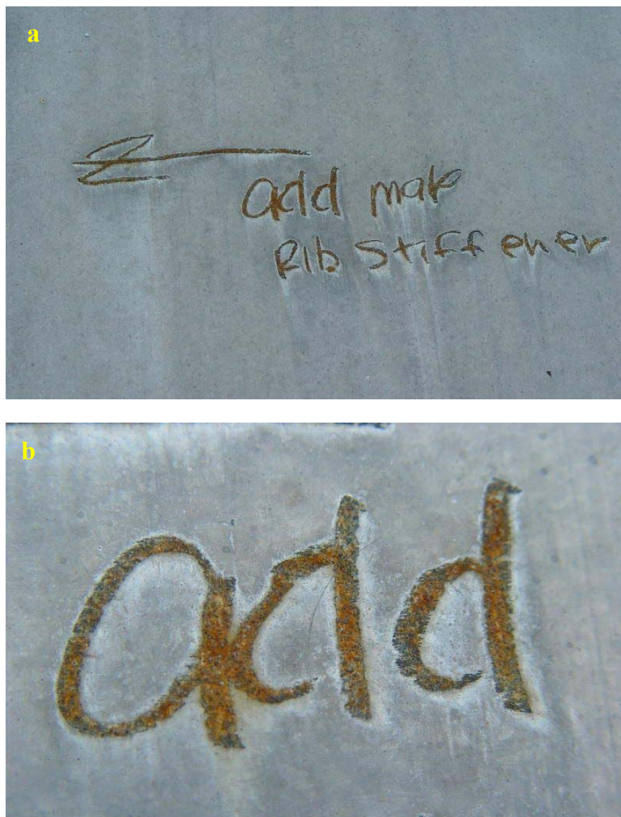
Figure 29. Photographs of pencil mark corrosion on galvanized steel sheet (a), and a magnified view of the mark (b).
