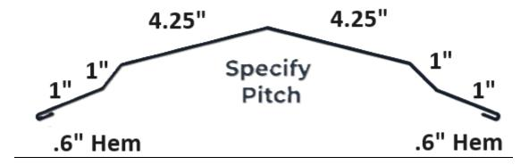
Snap a chalk line when installing your ridge cap. This allows you to keep your ridge peak in alignment with your roof peak as well as delineating where to place your closure strip if desired. When you screw through the kicker, closure strip, and into the rib of the panel make sure not to "Smash" or "Flatten" the ridge down while securing it to the panel.
