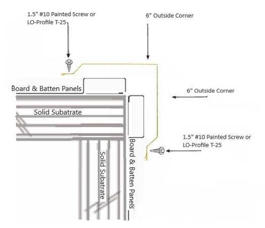
It is always a good idea to "dry fit" a corner before fastening it into place . Checking to insure the corner is square with the corner of the structure.
