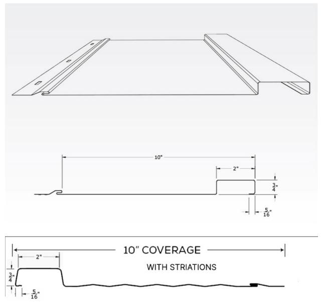
The Board & Batten product is a beautiful choice for siding in a residential environment. A solid substrate is required when installing this product.
