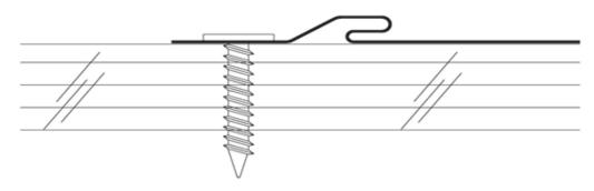
When fastening panels, it is important that you do NOT over "tighten" them. Over tightening will not allow the panel to expand and contract.
