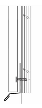
Drip Cap helps direct water away from door and windows openings. It can be used as a transition trim over rock, brick, and stone. Fasten with pan head screws or trim nails.
