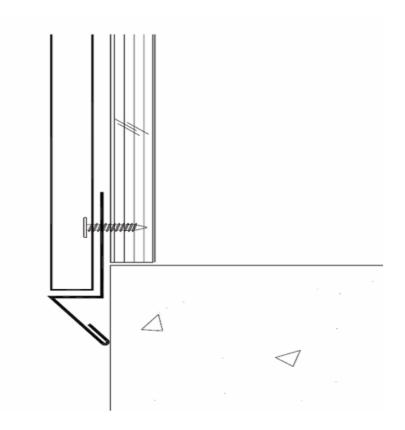
Rat guard or Square base should be used as a trim to seal between the sidewall panel, the concrete, and substrate. Its main purpose is to help with moister and rodent control.
