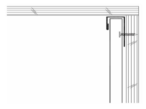
Use J trim to terminate into wooden soffit, doors, windows, and trimming around vents. When installing J – channel make sure that you leave enough room to allow for expansion and contraction.
