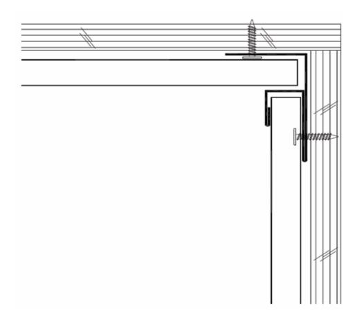
In terminating the Board & Batten into a soffit panel, the F&J trim will finish the edges and provide a closed edge for the soffit and sidewall panels.
